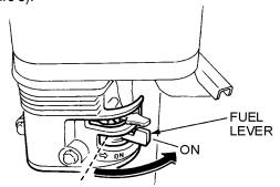
Figure 8. Fuel Valve Lever
